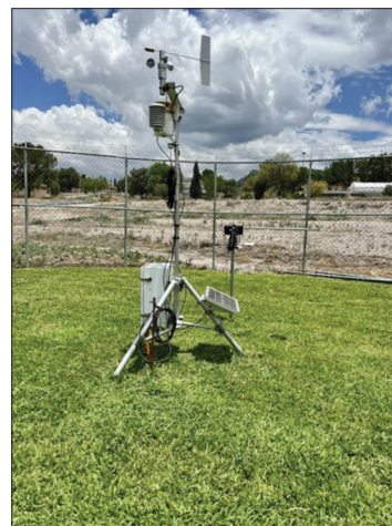
Figure 1: Automated weather station (Campbell Sci., Logan, Utah, USA) to obtain the meteorological variables for determining the FAO Penman-Monteith reference evapotranspiration
