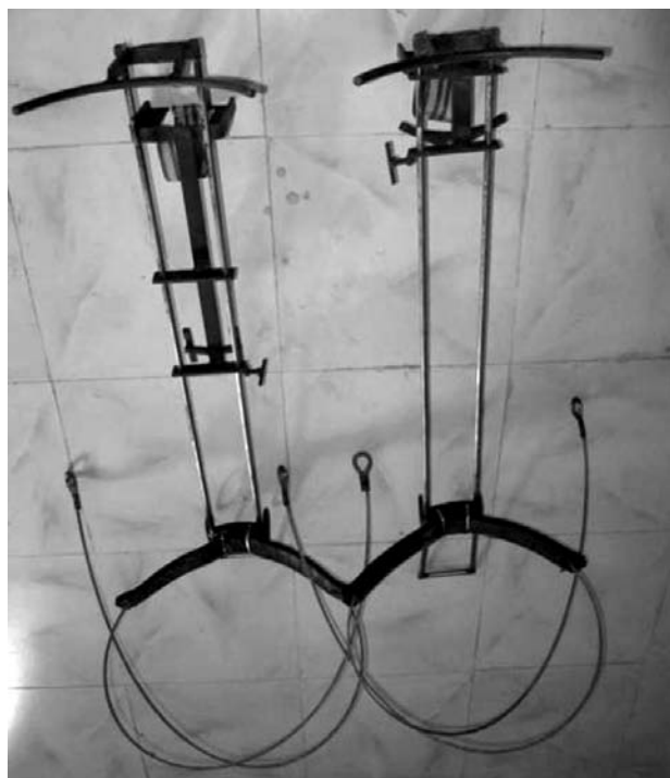
Fig. 1. Standing type or manually operated paddle type (tree walker)
